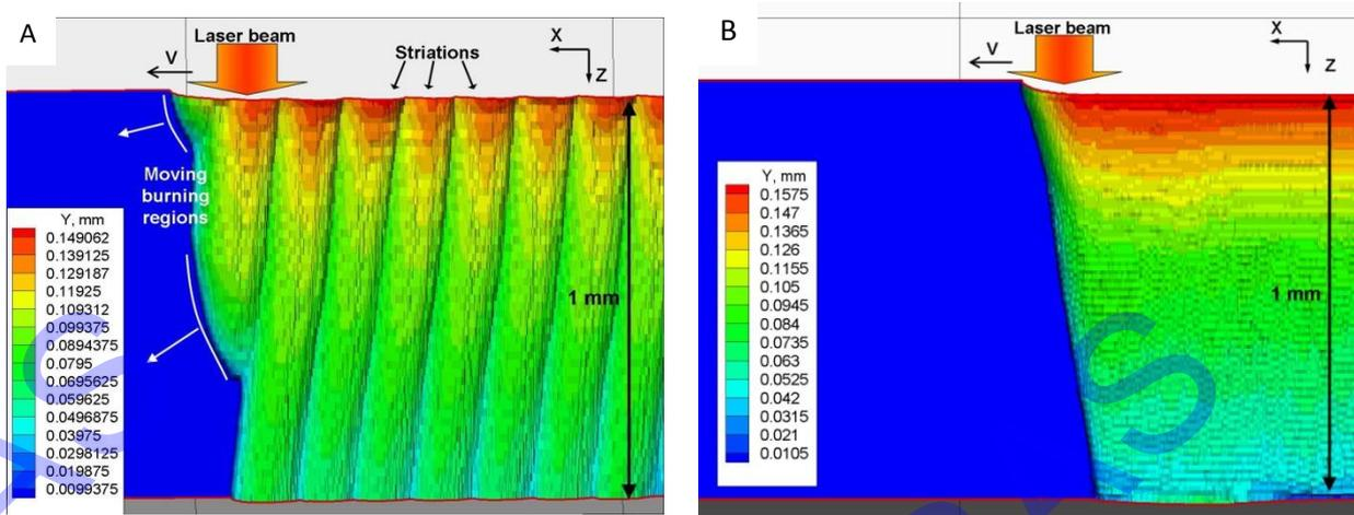
Cut surface profile. Cutting speed: A- 20 mm/s; B- 40 mm/s
