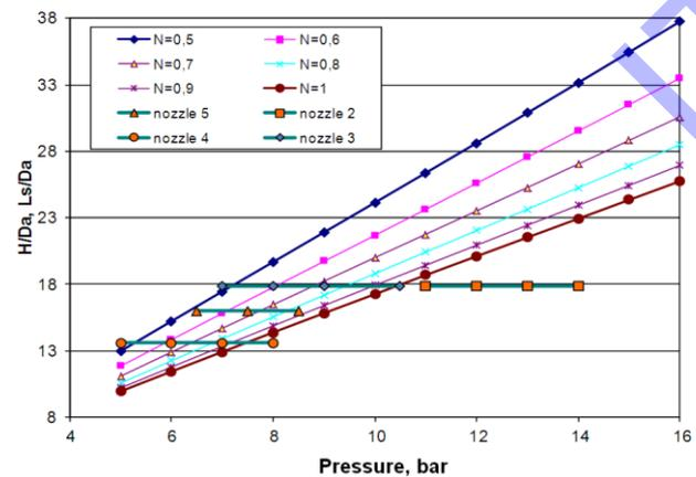
Calculated and experimental values of the dimensionless sheet thickness, and length of the supersonic part of the oxygen jet normalized to the nozzle critical diameter versus the pressure for different jet pressure ratios and nozzle geometries
