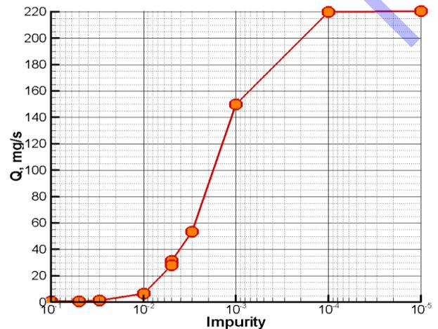
Reaction rate on the cut front versus the initial content of the inert impurity in the oxygen jet
