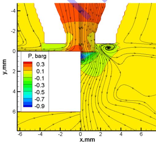
Pressure field and streamlines of oxygen flow inside cut kerf in the case of oxygen purity 99.99%.
