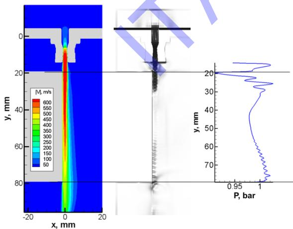
Supersonic jet flow of oxygen in the plane of symmetry of the channel geometrically similar to the cut obtained by laser-assisted oxygen cutting: gas velocity; gas density gradient; pressure on the leading edge.
